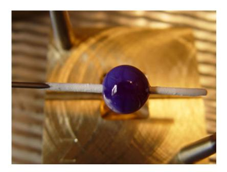
Step 4: Gently marver the fattest part of the round bead. This can be done with any marvering tool, or right on the corner of your new brass ZooziiPress. This gives the glass the basic desire to move into the corners of the press.
