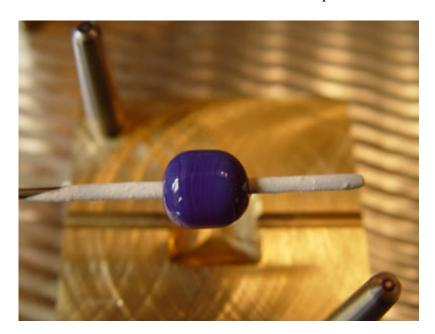
Step 5: Now you are ready to heat that squatty tube to the point that it is pliable, but not so that you loose the basic shape. Then press. This is what it will look like when you remove if from the press.
