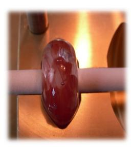
Heat and press. You want to be sure when heating that you do not get the glass hot enough that it starts to widen along the mandrel groove. This happens because the glass near the mandrel and the glass further from the mandrel both get to the melting point, causing both parts of the bead to want to merge together. At this point the glass is trying to form into a ball, which you do not want. So keep the glass near the mandrel warm, while the outer glass is getting hot. Then press.
