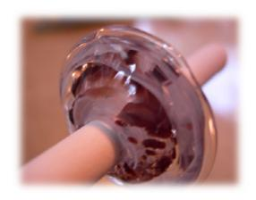
After your initial press, you will add glass along the narrow edge, only. Add there, even if you are missing glass along the edges. The reason to add only in the center is that when it's heated and pressed, the glass be pushed down and out into the press, which will fill in wherever the glass is needed. If you add where you think it's lacking, you will need to fight to keep the glass in the press.
