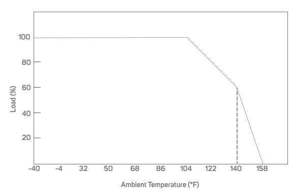
To extend the life of your driver, refer to the derating curve and derate according to the temperature.
