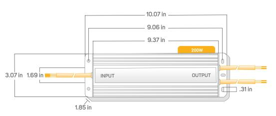
Input black and white wires to be connected to AC. Green wire to be connected to ground. Output red and black wires to be connected to LED lighting.
