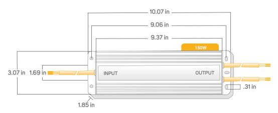
Input black and white wires to be connected to AC. Green wire to be connected to ground. Output red and black wires to be connected to LED lighting.
