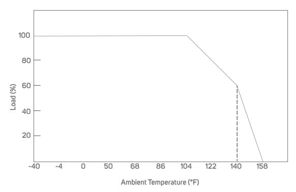
To extend the life of your driver, refer to the derating curve and derate according to the temperature.
