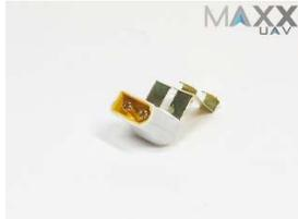
The adapter clip is easy to insert in the main battery. Insert the battery as usual and you will have a standard XT60 connector sticking out. The main battery is 4S LiHV, so you will need to use 4S LiPO or LiHV batteries. You can use any brand, size or capacity – just make sure they fit on the quad.
