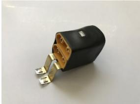
The adapter clip is easy to insert in the battery connector. Use pins 2/3 and 5/6 from the left (counting only the metal pins). Make 100% sure this is correct! Insert the battery as usual and you will have a standard XT60 connector sticking out. The main battery is 3S LiHV, so you will need to use 3S LiPO or LiHV batteries. You can use any brand, size or capacity – just make sure they fit on the quad and are not too heavy.
