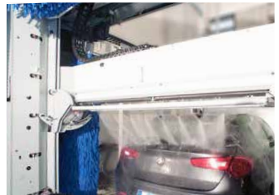
Vertical dryers full height
