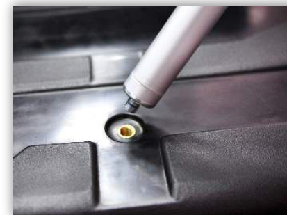
4. Screw the poles into the case
