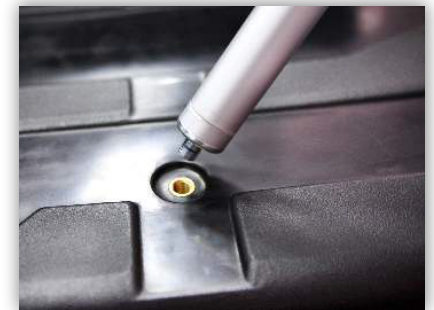
4. Screw the poles into the case
