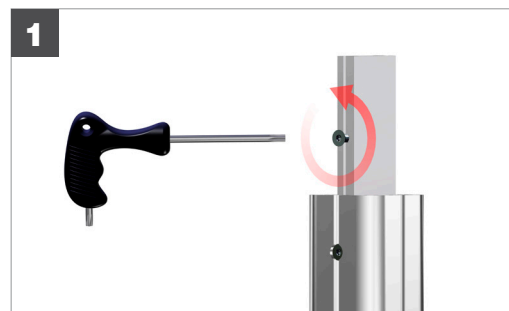
1 REMOVE TORX SCREW FROM LOCATING BAR AND SET ASIDE
