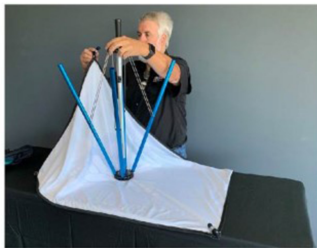
Insert plugs on all four corners
