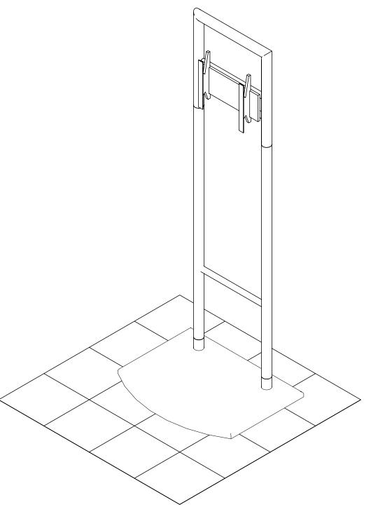
Step 1. Connect the plates to the base using four screws per plate as shown in the attachement detail below. Assure holes on tubing are facing inward.
