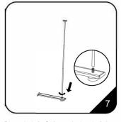
7.Insert both the 3-piece-poles into the hole of the base, then fix the other end of the base unit Connect the two basic unit with a
