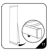
11. The unit can be levelled by adjusting the threaded feet at the bottom of the base unit.
