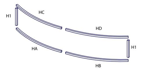
Base support framework — please note the forward curves break along the center. Door attaches to upright #2
