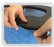
8. Pull graphic taut and angle and tuck gasket into channel in edge of foot. Insert graphic gasket all the way around.
