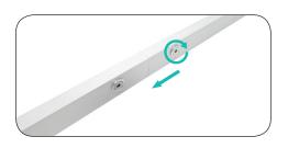
**c.** Then slide the other extrusion onto split connector. Make sure extrusions are flush and tighten the screw to secure connection.
