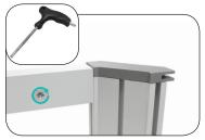
**d.** Connect the top extrusions together and use torx key to tighten.
