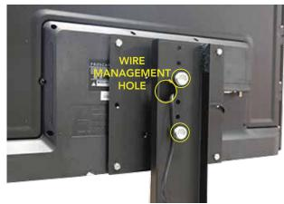
STEP 5: Next, lift your monitor up to desired height and screw the monitor into place.
