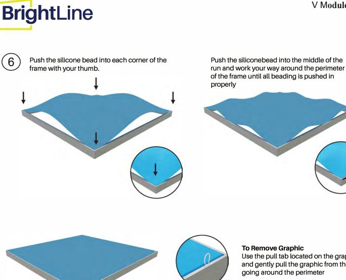
**To Remove Graphic** Use the pull tab located on the graphic and gently pull the graphic from the frame, going around the perimeter
