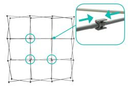
**c.** Close frame by pushing the outside of the frame until male and female ends connect.
