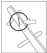
2 Start with smaller stand alone pole section and guide down into both slots on the back of the unit as shown at left
