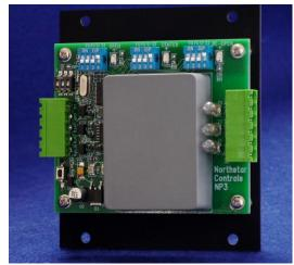
The NP3 has been specifically designed and engineered for use in the Parking/Access Control industries and is designed for use where open, safety and exit loops are used. With standard operations including compatibility with all radio controls and more, the NP3 covers your low power, plug-in detection needs.
