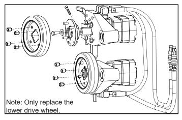
Figure 7. Mount the Drive Wheels
