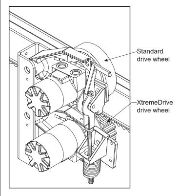
Figure 9. Assembled XtremeDrive System
