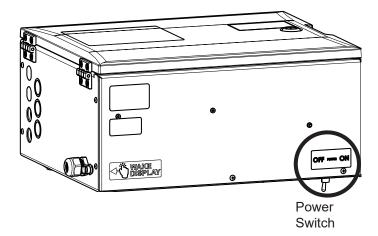
Figure 2. Set Power Switch to OFF
