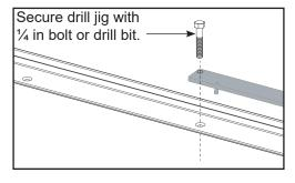
Figure 4. Align the Next Set of Mounting Holes
