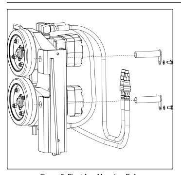
Figure 6. Pivot Arm Mounting Bolts
