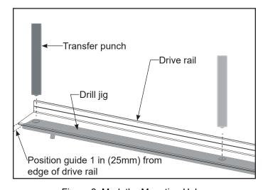
Figure 3. Mark the Mounting Holes
