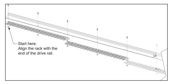
Figure 5. Mount the XtremeDrive Rack
