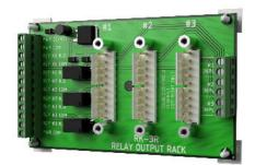
Many vehicle detectors are designed to be plugged into a rack including some of the more popular Diablo Controls models. In those installations where a large rack is not available, Diablo Controls has designed a mini rack. The RK-3R is designed to accept up to three plug-in vehicle detectors on one side and accept the appropriate wires through the terminal block on the other. The entire mini rack is supported by four adhesive standoffs that attach anywhere in the cabinet.
