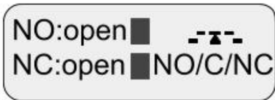
Figure 8: Relay test screen shown without a relay connected (both NO and NC terminals are 'open').
