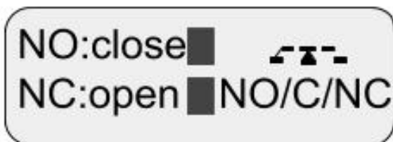
Figure 10: Relay test screen shown in which the relay NO terminal is measured as 'close' (shorted) to the relay COM terminal indicating that the relay is in the energized state.
