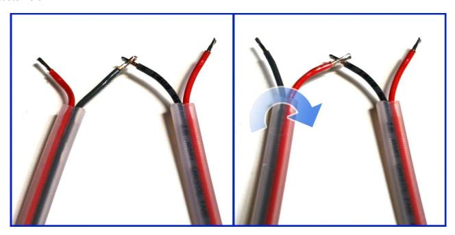
If you try to take advantage of loop phasing and discover that the loops are detecting the gate – it may mean that the loops were not properly phased. Don't worry, you don't need to pull up the loops and re-install them. You just need to take one lead-in and flip it over. Doing this will change the direction that current flows through the loop and cause the polarity of the loop to change. Hook the loops back up to your detector and see if the gate is still being detected.
