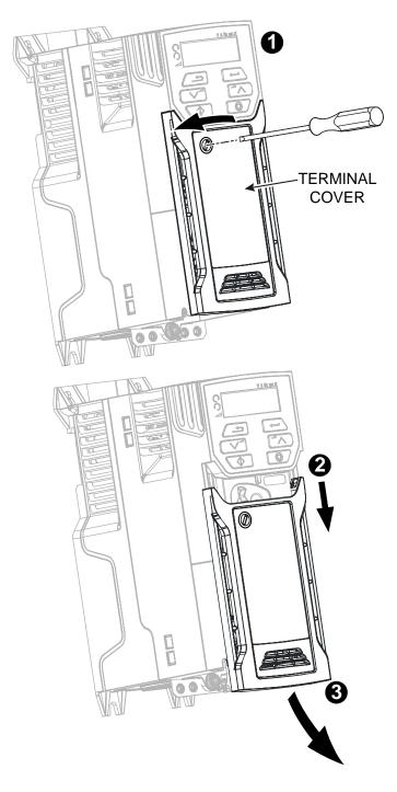
Figure 4. Remove VFD Terminal Cover
