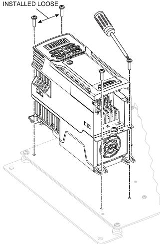
Figure 6. Mounting VFD to Control Box
