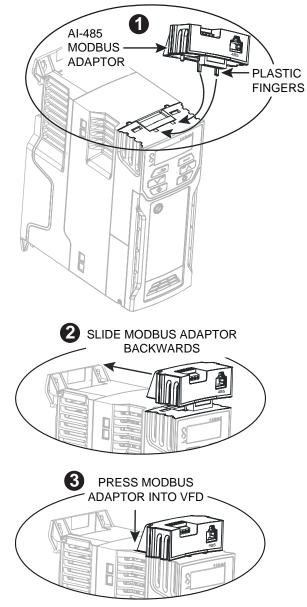
Figure 5. Connect AI-485 ModBus Adaptor to VFD
