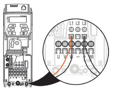
Figure 9. Connect Input Power and Transformer Wires to VFD 6. Use Torx driver to connect ground wire to ground terminal strip and grounding point. See Figure 10.
