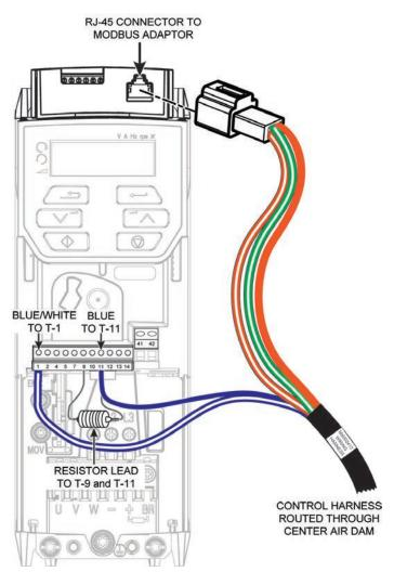
Figure 7. Connect Control Harness Wires to VFD
