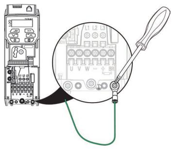
Figure 10. Connect Ground Wire to VFD Terminal Strip
