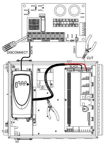
Figure 2. Disconnect Gray, Red, and Black Wires
