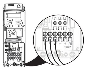
Figure 8. Connect Motor Wires to VFD
