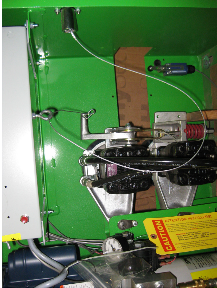
SlideDriver interior showing cable release mechanism
