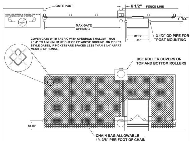
Figure 2. Post Mounting Specifications
