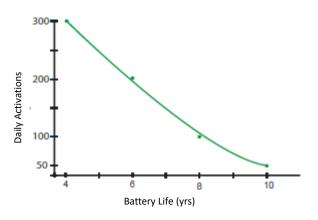
Note: Battery life is dependent on many factors, including daily activations, time used per activation, radar range and external conditions.
