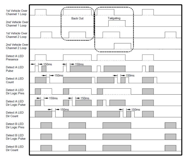
Figure 9: Detect LED Indications During Directional Logic
