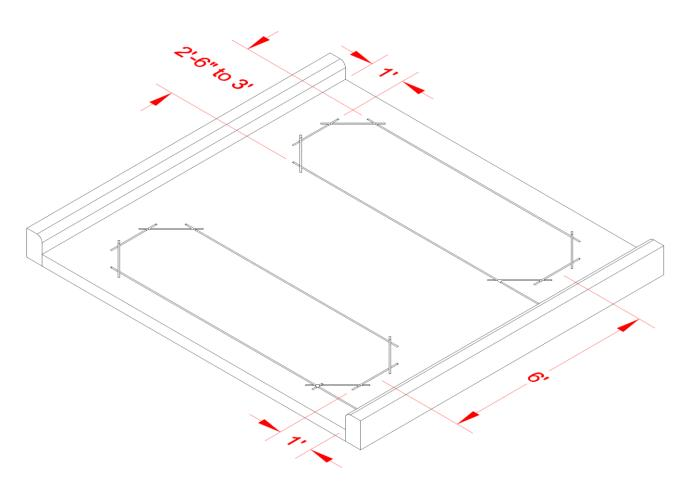
Figure 11: Loop Placement
