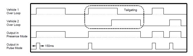
Figure 3: Mode 0 - Two Individual Channels with Pulse or Presence
