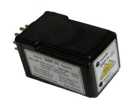
Fail Safe Operation - The DSP-11 series of detectors are designed to be "Fail Safe" in their operation. The detector will output a "Detect" (contact closure) for a "Failed" loop condition OR a loss of power to the detector. This "Fail Safe" detector should always be used on "safety" loops.
