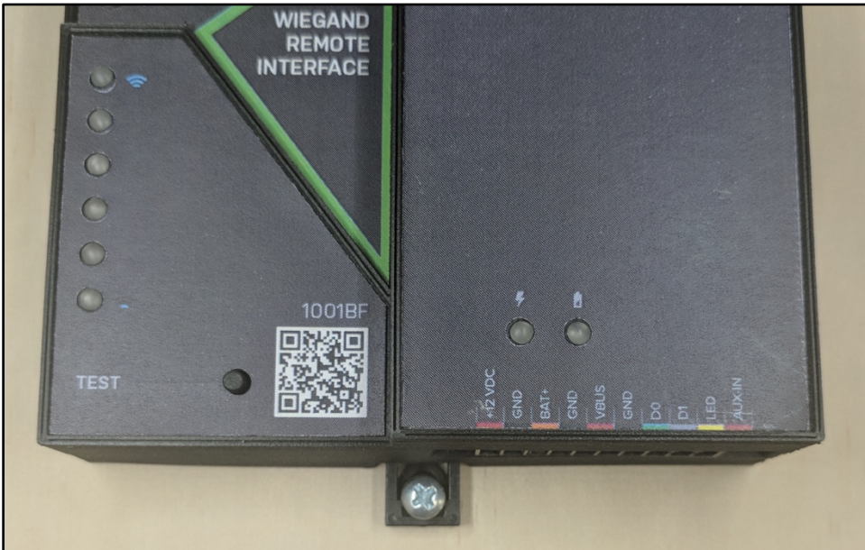
Figure 8: The bottom screw is shown mounted through the black DIN clip to the wall:
