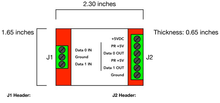
Data 1 IN - Wiegand Data Input 5-24 VDC Ground - Input Ground Data 0 IN - Weigand Data Input 5-24 VDC +5VDC - Input, regulated 5VDC @ 30mA
