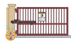
DO NOT install next to sprinklers or any area that may expose the bottom of operator to water.
