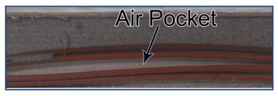
air pockets. Luckily preventing issues with air pockets is as easy as switching to a 3/16" or larger saw blade. Don't let all your hard work go to waste, using a wider saw blade can make your loop installations less prone to failure. Protect your reputation and prevent the unneeded, and hard to diagnose service calls air pockets cause.
