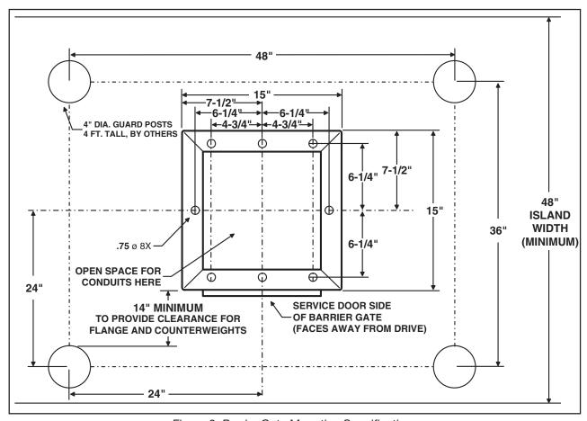
Figure 2. Barrier Gate Mounting Specifications
