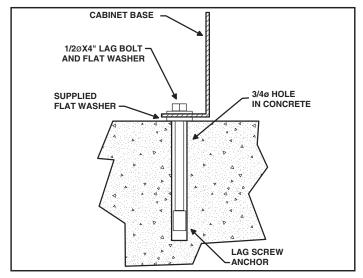
Figure 1. Concrete Lag Anchor Detail
