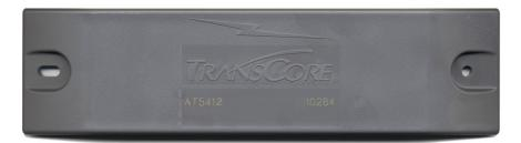
The AT5412 Harsh Environment Transportation Tag is a half frame, beam-powered tag used in 915 MHz radio frequency (RF) band applications with TransCore Amtech-brand and TransCore Encompass multiprotocol reader systems. It is packaged in a factory-sealed case, which makes this tag ideal for mounting on vehicle chassis, intermodal containers, or in any environment requiring a durable, weatherproof tag.
