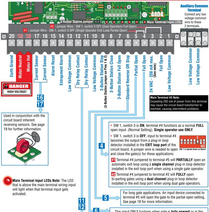
Operation of relay is dependent on setting of SW 1, switches 4 and 5. See page 16 and 17 for DIP-switch function descriptions.
