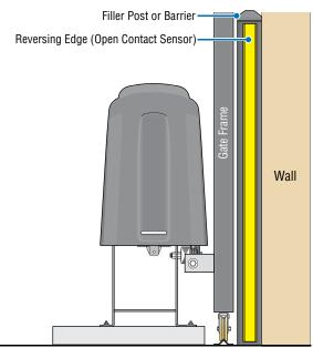
A filler post or barrier may need to be installed between the gate and wall area to reduce the distance to 2 1/4" **or less**. A reversing edge should be installed on the post or barrier for safety (See pages 2 and 3 for more information).
