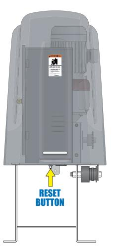
If the cause of the alarm cannot be corrected, shut-off power and **DO NOT** place this operator back into service until the malfunction can be identified and **CORRECTED**.
