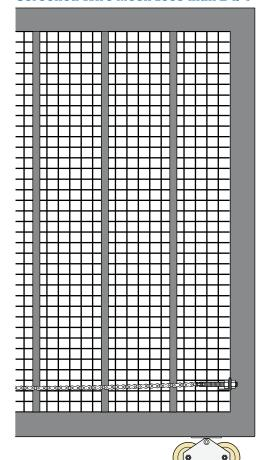
DoorKing recommends installing screened wire mesh on the **ENTIRE** gate **AND** and on that portion of the adjacent fence that the gate covers in the open position. (See above).
