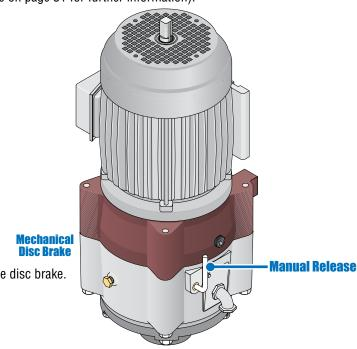
NO adjustment is needed for the disc brake.
