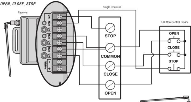
Refer to your commercial door operator or gate operator wiring diagrams for instructions on connecting two or more 3-Button control devices.
