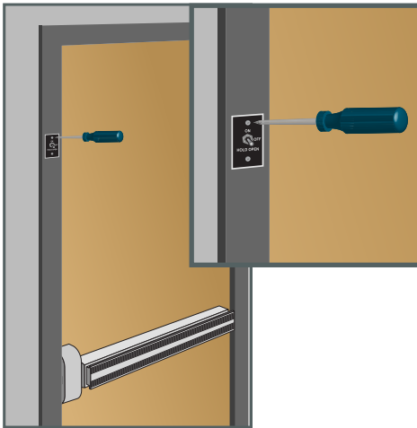
ON / OFF / HOLD OPEN Switch installed
