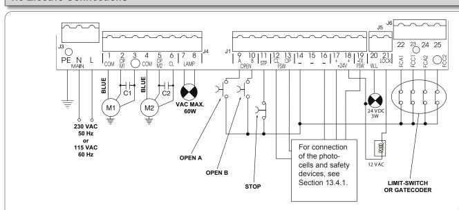
NB: Capacitors are supplied with the operator.
