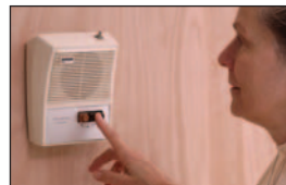
intercom model 1504 combines the keypad with an intercom substation that can be used with some existing intercom systems
