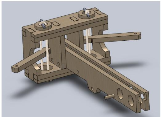
24. Assemble the pawl and its axle by sliding the pawl and 3 of the windlass drum pieces onto the pawl axle as shown.
