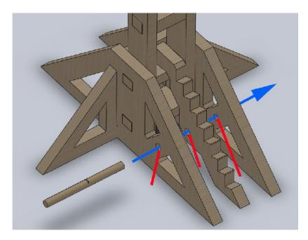
6. Assemble the "breech" with the parts shown below. Use 3 of the three line marked dowels to temporarily bind the 3 wooden parts together. Once you have them put together, leave equal lengths sticking out of either side on the front two dowels. But the rear dowel will end up flush on the right side. GLUE NOTE: **Do not glue these parts yet** as you may need to adjust them later.
