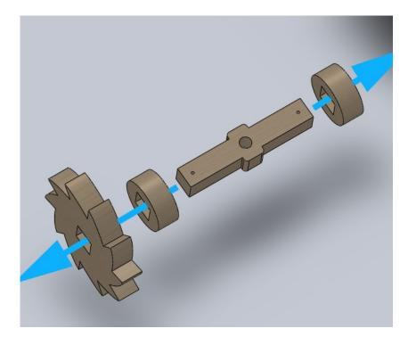
30. Fix the ratchet gear onto the axle using a metal rod.
