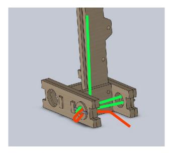
You want to keep the string under tension as you wrap and try to not let the string stack over itself. Rather, you want each loop where it passes around the steel bar to be separate. In the illustration below, the first loop is green, changing to red as it passes back through the washer closest to you, then to blue. Only 3 loops are shown for clarity. **Make 4 to 5 loops.**
