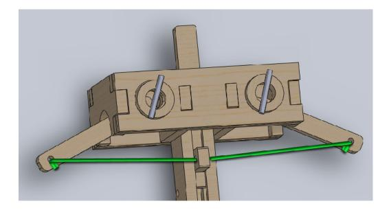
39. Slide the trigger slide forward until it rests against the firing rail slide. Then run the end of string from trigger slide through the hole in the windlass axle. Leave a bit of slack and tie a simple knot in the end and trim the string.
