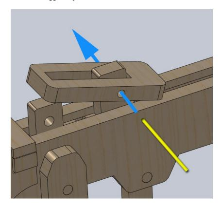
Trim the excess ends of string, and you are finished with assembly of the Desktop Ballista
