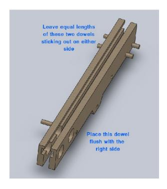
7. Add the frame inner pieces to the assembled breech as shown, inserting the dowels through the holes in the frame inner parts. GLUE NOTE: If you are using glue, apply glue to areas shown by red indicators. Apply only a small amount to the dowels. Once together, ensure that the 2 front dowel ends are flush on both sides but the rear dowel is only flush on one side.
