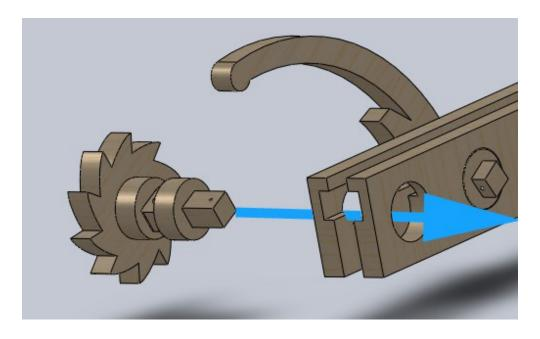
32. Add the windlass crank handle onto the end of the windlass axle and fix it in place with a short metal rod by bending the ends around the axle as you did on the side with the ratchet gear.
