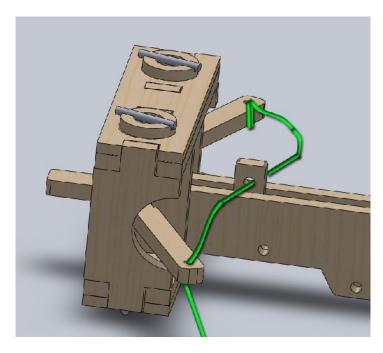
38. Then pull the string and tie it onto the other arm (2 turns and half hitch will work okay). You should end up with a string that goes pretty straight across. Some slack is okay, but it should be minimal.
