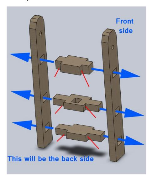
2. Insert the completed mast into the side feet parts. IMPORTANT: The notches in the side feet parts (part number 5) go to front of the ballista. Part number 3, the middle horizontal part in the mast has the hole closest to the back side of the ballista. If part number 3 faces to front of ballista, then the elevation ramp (part number 7) will not align properly. See step 4 to see how that part attaches. GLUE NOTE: If you use wood glue, the red arrows show the areas to apply wood glue.
