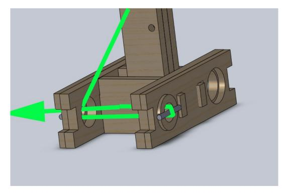
18. The color of the string in the illustration changes from green to red to show the transition from loop number 1 to loop number 2. This looping path is repeated to create 4 to 5 total loops.
