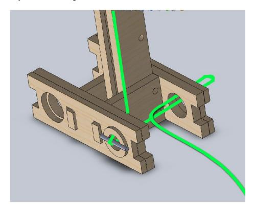
15. Thread this loop through another round washer on the other side of the frame as shown.
