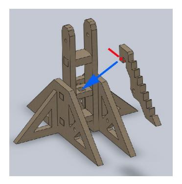
5. Insert the dowel with the one line mark (longest of the dowels) as shown to fix the elevation ramp in place. If you do not have the hole in the middle horizontal part of the mast assembled correctly, the dowel holes for the elevation ramp (part number 7) will not line up.GLUE NOTE: If you are using wood glue, place as shown by red lines into the dowel holes.
