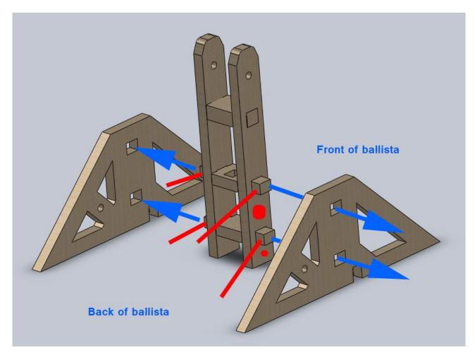
3. Insert the base foot front as shown. GLUE NOTE: If you are using wood glue, add wood glue as shown by areas in red.
