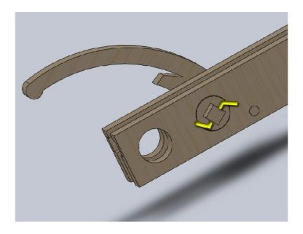
29. Assemble the windlass axle as shown using the ratchet gear, windlass axle and 2 windlass drums. Note the direction of the ratchet gear's teeth.
