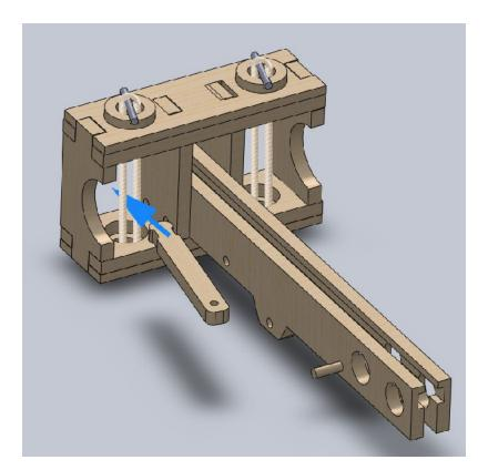
23. Turn the washer/steel bar so that a twist is created into the skein (string), causing the arm to rotate to the outside of the frame. Turn about 45 degrees at a time on both top and bottom washers, until the arm is against the outer frame.
