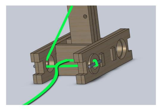
17. Then thread the end of the string through round hole in the washer and over the steel bar
