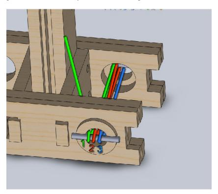
19. In the illustration below, the different colors are removed and only a single color is used to show 4 loops with the end of the string finally coming through into the inside of the frame where the taped end is. You will join these two ends with a square knot. Do not cut off the excess string ends yet. You can remove the tape.
