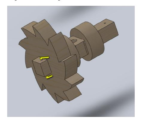
31. Insert the assembled windlass axle into the breech.
