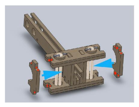
22. Insert an arm into the skein center as shown.
