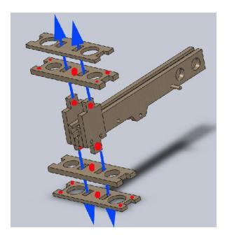
9. Stand the frame and breech assembly on end as shown
