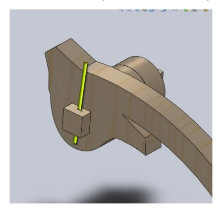
26. Bend the ends of the metal rod to hold the pawl onto the end of the pawl. Needle nose pliers are best for this, but the metal is soft enough to where this can be done by hand.
