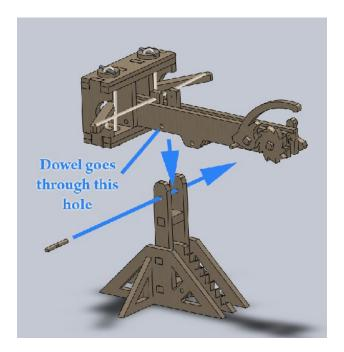
41. Mount the elevation stake to bottom of the breech using a dowel marked with 2 lines.
