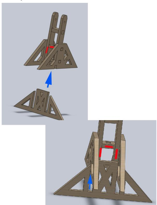
4. Insert the elevation ramp piece into the base as shown. If you do not have the hole in the middle horizontal part of the mast assembled correctly, the dowel holes for the elevation ramp (part number 7) will not line up. GLUE NOTE: If you use glue, place as shown by red.
