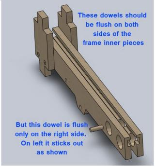
8. Add the frame horizontal pieces as shown. Note that the outside most pieces will be thinner material and will have a larger diameter circular hole than the inner most pieces. GLUE NOTE: If you are using glue, add to areas indicated in red.
