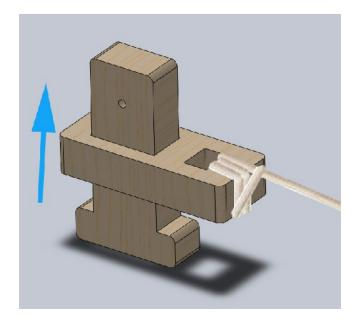
35. Insert the trigger horizontal slide into the breech from the front.
