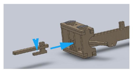
37. Using the remaining short string, tie through the hole in the arm on one side, then through the firing rail slide then into the other arm's hole. Don't trim the excess off the first arm's knot yet.
