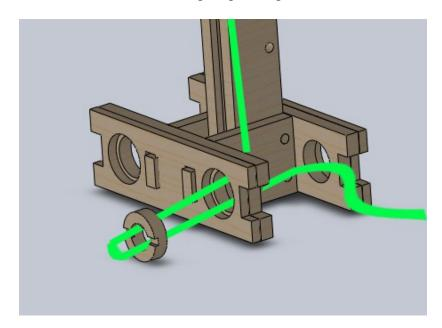
12. Then insert a steel bar through the loop.
