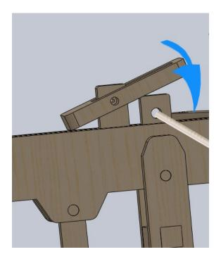
With the trigger over the firing rail slide, lowe the pawl to re-engage the ratchet gear. Then rotate the windlass crank handle as shown. This will pull the trigger toward the back of the ballista, dragging the firing rail slide with it. This will look much like drawing a bowstring.
