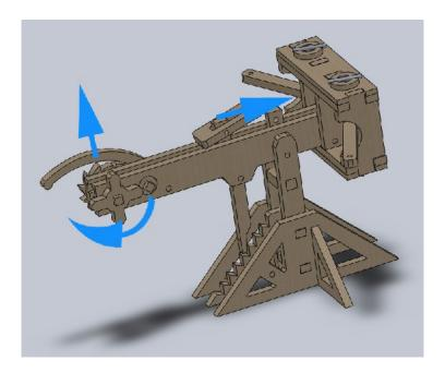
Lower the trigger's front edge down onto the firing rail slide
