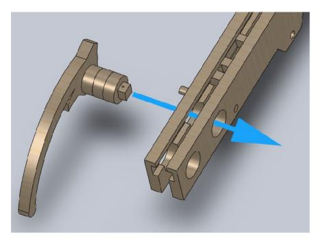
28. Insert another metal rod into the pawl axle on the other end in order to hold the windlass drum onto the axle. Note that you want to bend the wire so that the ends overlap the windlass drum and the breech part as shown. If you only bend around the axle, the entire pawl axle assembly can still slide out to the left.
