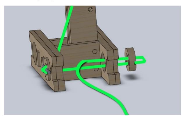
16. Insert another steel bar through the loop and tighten the string to pull the washer and steel bar into the frame as you did on the other side.
