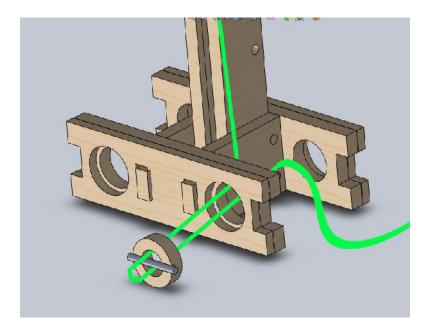
13. Gently pull the string until the washer and steel bar are pulled into the frame hole. Maintain tension on the string to keep the washer and steel bar in place as you do the next steps. You want to keep tension on the string throughout this process.
