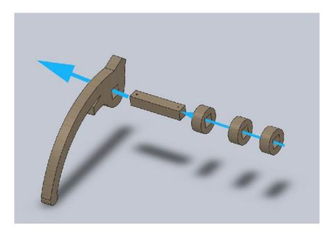
25. Insert one of the short metal rods into the pawl axle hole at end where the pawl is located.
