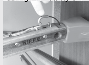
Locking Pin - Safety ON
