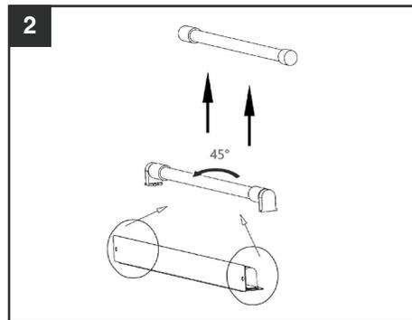
3. Install new UV lamp. Gently place new lamp in place, firmly turning 45° in opposite direction of removal. Place UV lamp cover and tighten screws.
