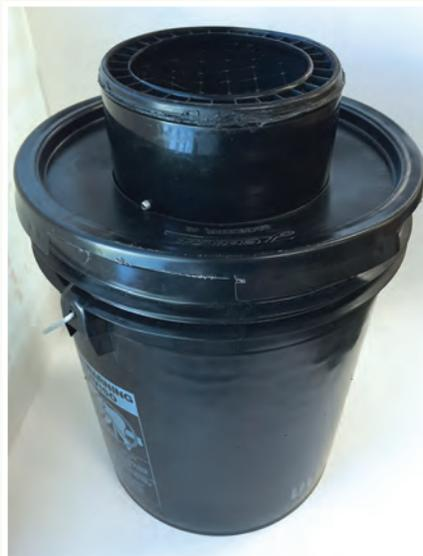
Figure 1: The original AGO was hand built by researchers at the CDC using off-the-shelf materials, including a 5-gallon bucket, a plastic paint can, and multiple types of mesh.
