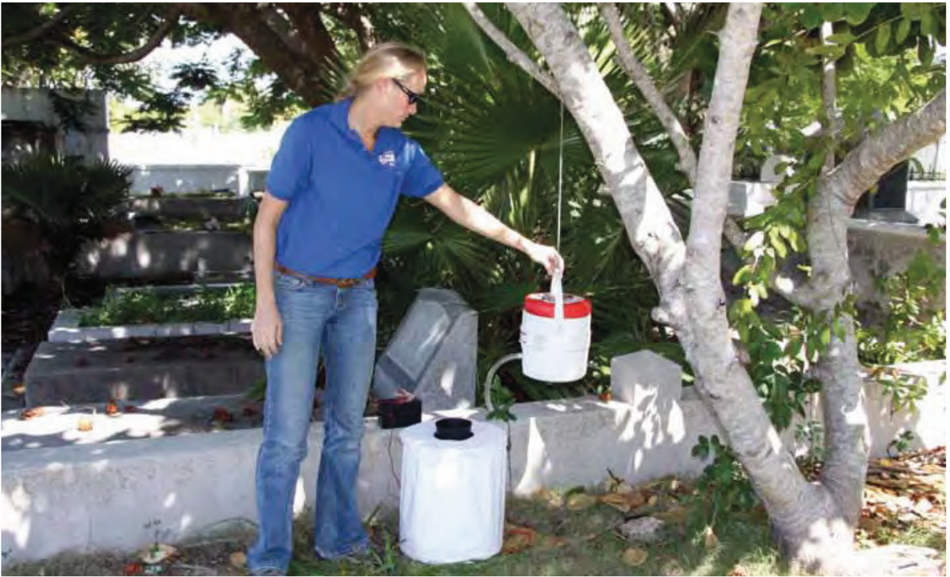
Figure 4: FKMCD Deputy Director Andrea Leal sets up a BG-Sentinel Trap with dry ice to collect Aedes aegypti .
