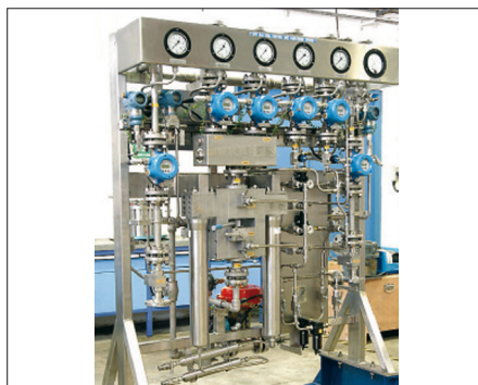
Filter station for the filtration of gases with STAUFF-3-way-selector ball valves for 250 bar / 3600 PSI and +200°C / +392 °F.
