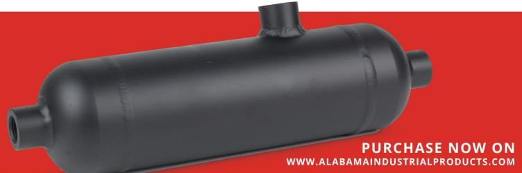
Condensate Pots are a form of protection for sensitive instrumentation components. They are design to collect foreign debris and accumulate condensate to help prevent damage to sensitive inline instruments. The bottom connection is able to serve as a drain port that can be equipped with one of AiP's ball valves.
